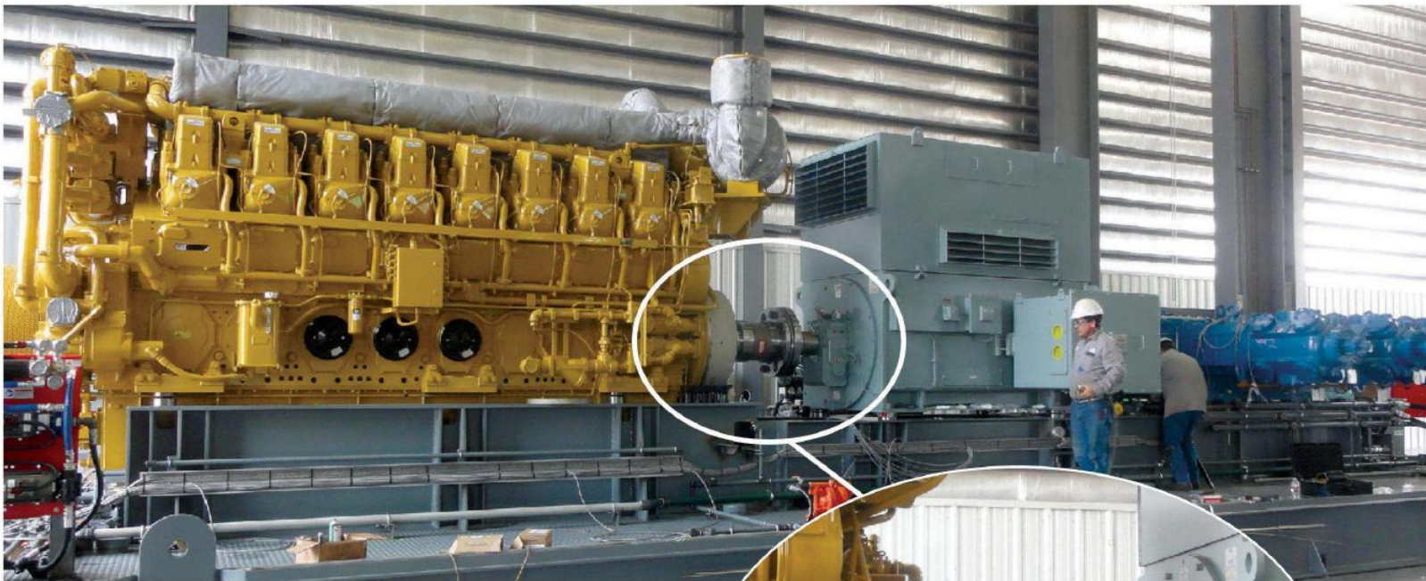
A typical dual-drive compression system features a natural gas engine, an electric motor, and an overrunning clutch.
