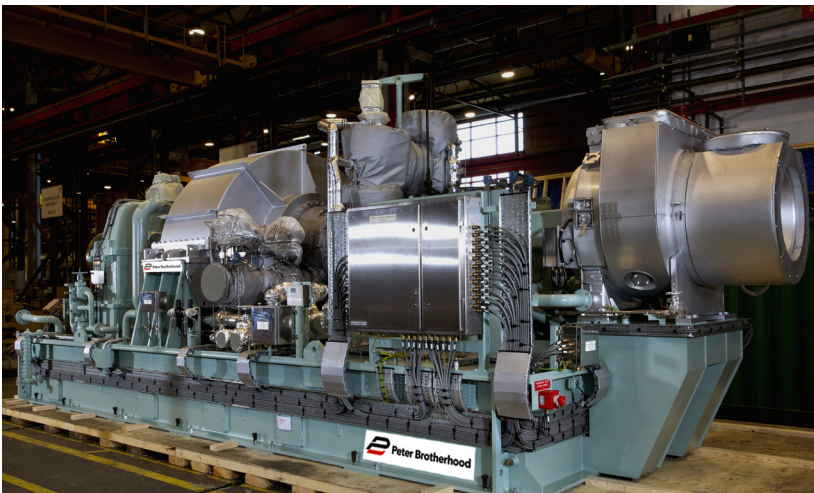
Figure 1. A skid mounted Peter Brotherhood waste heat recovery system like this one operates inside all Emma Maersk E-Class Series supercontainers (photo credit: Peter Brotherhood Ltd.).
